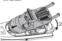
6. Turn the knobs as shown and finally lock the boat body.
